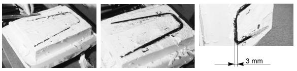
1.) Remove the foam entirely until the evaporator tube is visible. The evaporator tube should protrude 3mm.
